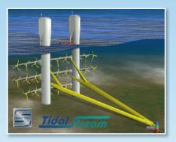
rotor blade has been developed and produced by Avantgarde Technologie GmbH for the SCHOTTEL Group using VAP® technology and process engineering support from Composyst GmbH. To limit the shearing forces that can occur at overspeed, the intelligent blade adjusts in shape to enlarge its pitch angle. This significantly reduces thrust augmentation and keeps the load exerted on the turbine and the supporting structure at a low level.
